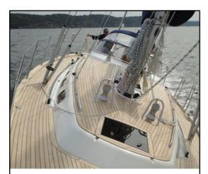
Clean deck design with stainless steel grabrails, large dorade vents and extra deck hatches
