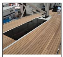
Clear decks with ropes led out of sight and flush-fitting hatches
